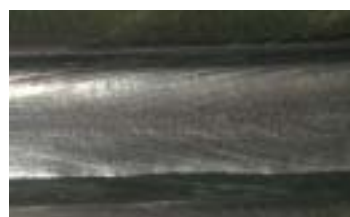
Figure 3. Typical smooth and flat weld bead surface appearance of SCW™ weld in duplex stainless steel.
