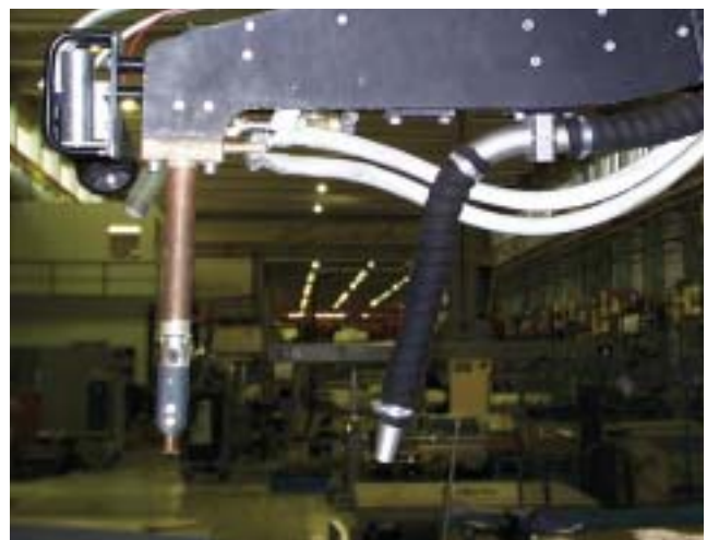
Figure 4. New compact SAW twin arc welding head.
