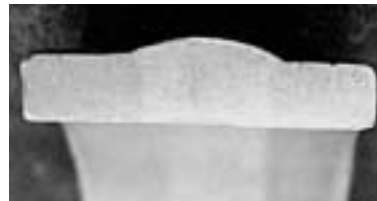
Figure 2. Weld appearance and macro of orbital weld.
