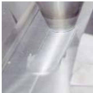
Figure 1. FSW process in a butt joint against backing bar.
