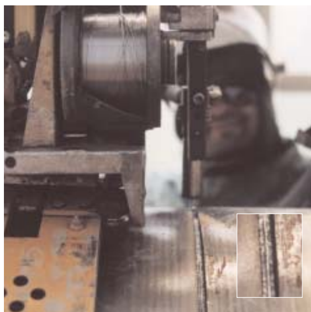
Figure 3. Root pass produced under CO 2 gas protection. Note the rim in the heart the weld, which is typical for CO 2 .
