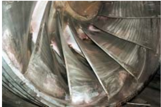
Figure 6. Section of a Francis turbine runner welded with the metal cored wire FILARC PZ6166.
