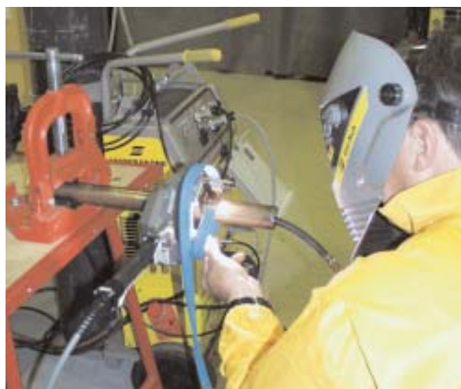
Figure 1. Test welding at ESAB Oy, Finland, using a Prowelder 160 power source and PRB 33-90 welding head.
